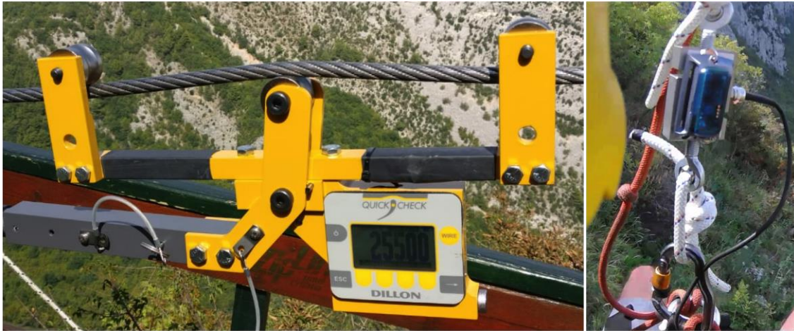
Figure 4. Tension force measurement due to static loading (left), force and acceleration measurement on the pendulum attachment point (right).
